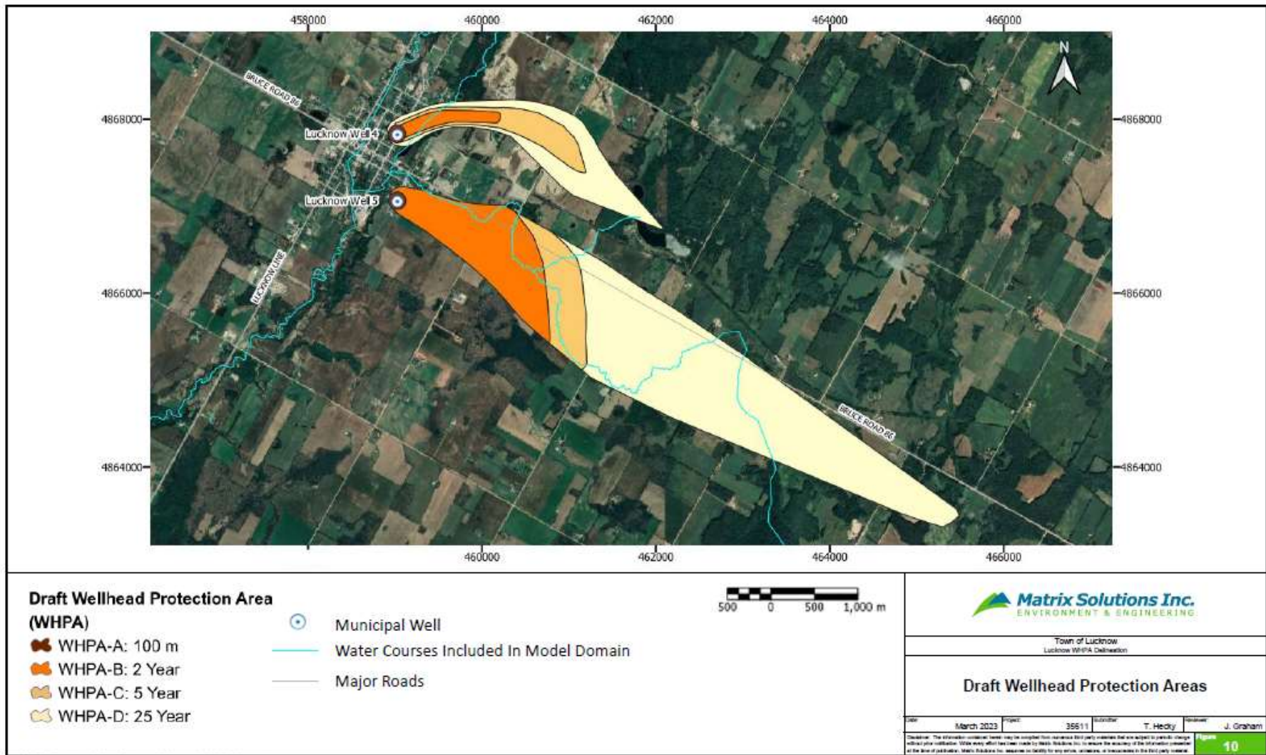
Figure 2: Draft Wellhead Protection Area. From Preliminary Wellhead Protection Area Delineation and Vulnerability Scoring Lucknow Well 4 and Well 5 , Matrix Solutions Inc. 2023
