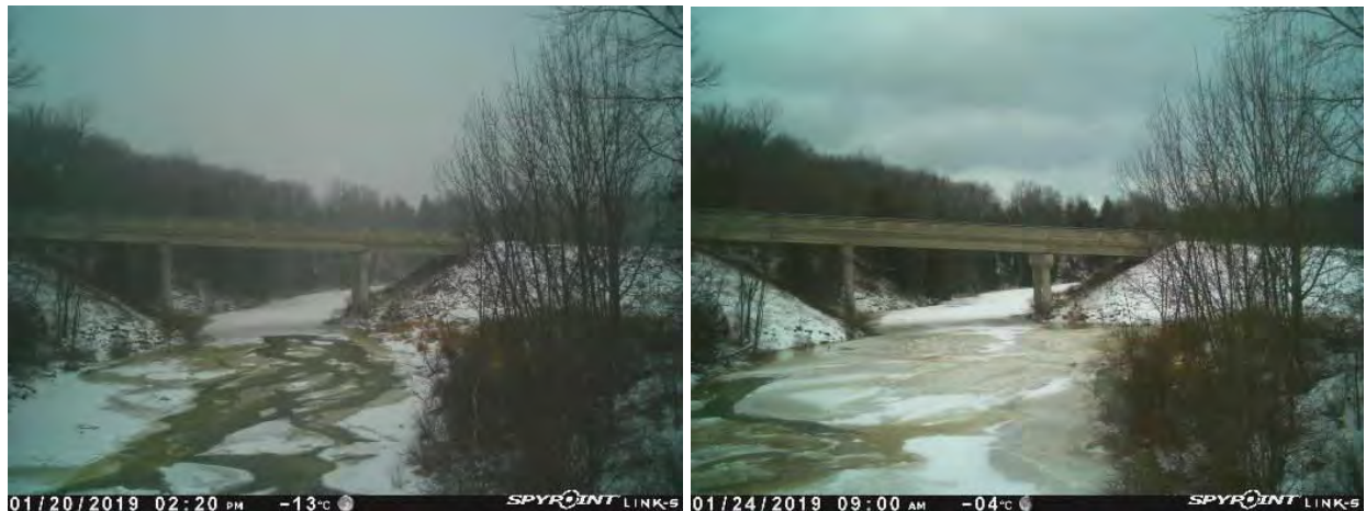
Figure 11. Sample photographs showing end of ice sheet cover and frazil formation (left); noticeable increase in water elevations (right)
