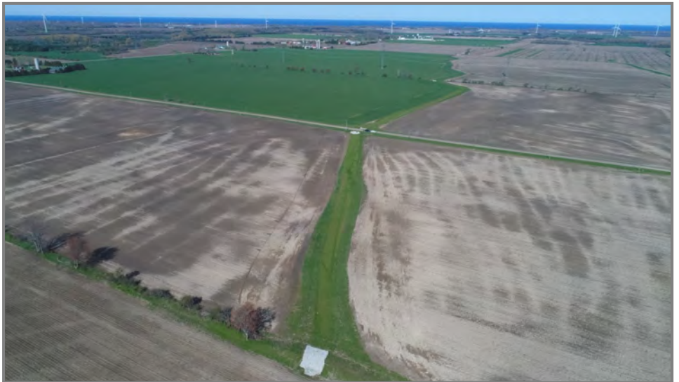
Aerial photos taken in the Garvey-Glen watershed show how construction of berms and grassed waterways keep water off the fields during rainstorms which protects the soil and keeps the water clean before it ends up in Lake Huron.
