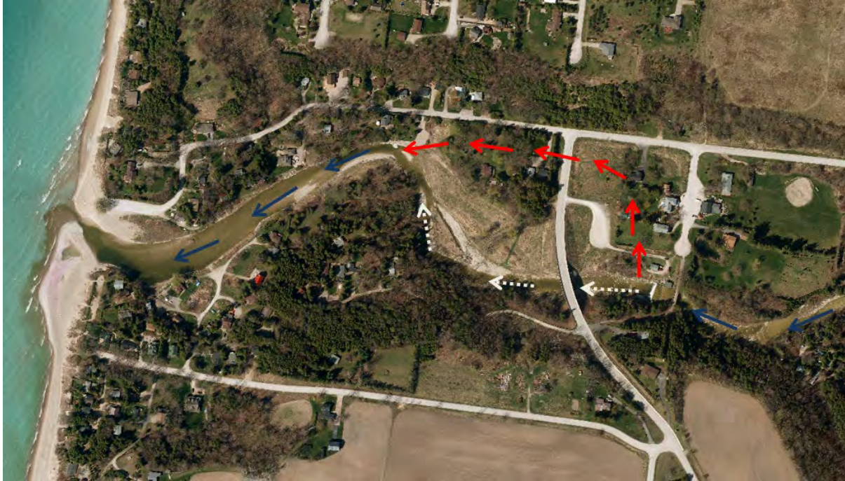
Flow path of flood waters during a frazil related ice jam at the Port Albert Fishway in 2016
